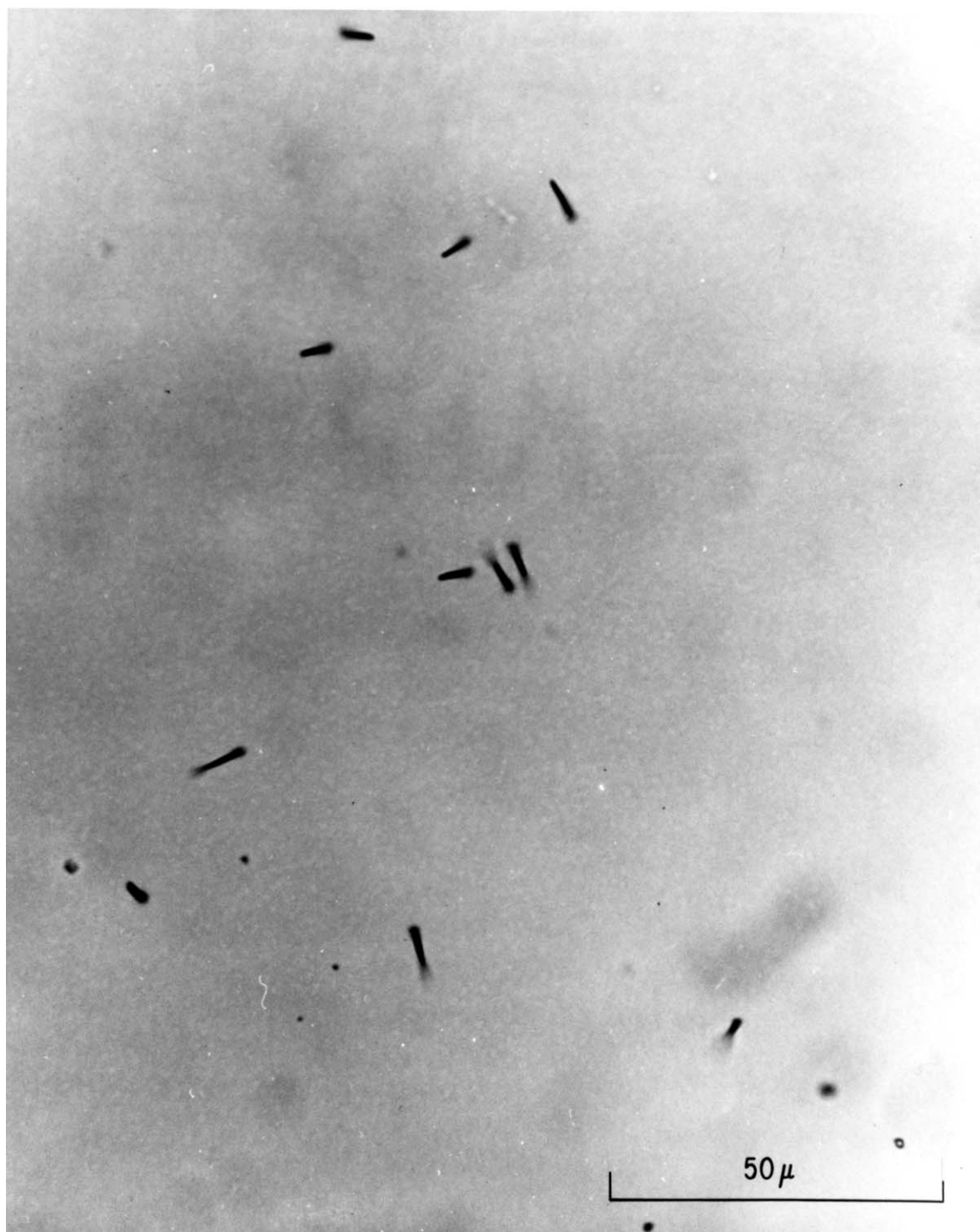
Figure 1 Mica was the first substance in which ^{238}\text{U} spontaneous fission tracks were identified by Price and Walker [2]. The tracks in this Madagascar phlogopite were revealed by etching in hydrofluoric acid. From Fleischer and Price [5], reprinted by permission of Pergamon Press, Ltd.
